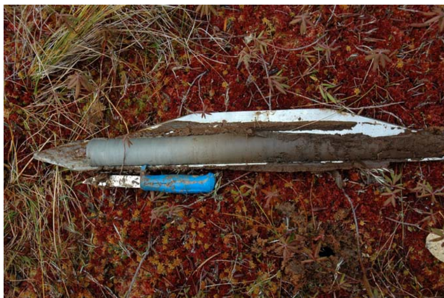
Figure 4. Extracted core showing transition between basal peat (R) and glacial lake sediments (L). The bluish-gray colour of the sediments indicates anaerobic (oxygen-poor) conditions.
